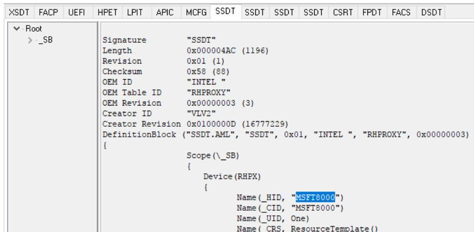
For the other Intel Atom platforms we tested, RHPROXY was not supported in the firmware, thus UWP application access to the microcontroller IO was not possible. Following the aforementioned guideline, one could add the support to the registry, but intimate knowledge of the hardware is required, which might not be possible in most cases. If you want to access GPIO, I2C, SPI, and UART from a UWP application, you will have to work with your hardware vendor to get support in the firmware.
