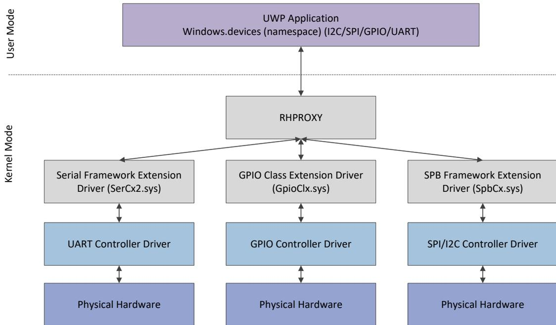
RHPROXY is a driver that shows up under the System Devices in Device Manger.
