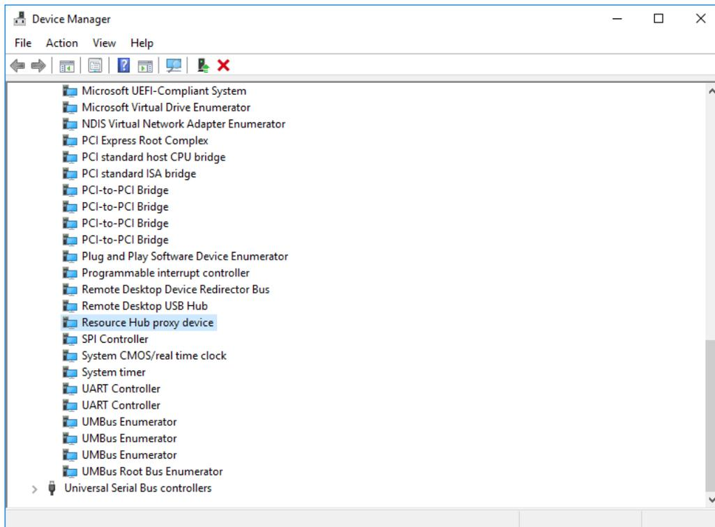
For the driver to load, the firmware must list "ACPI\MSFT8000" in the ACPI tables. In the Minnowboard Max, RHPROXY shows up in a Secondary System Description Table (SSDT). There are several options to check for RHPROXY support in your PC platform, the first is to install Windows 10 16299 and see if RHPROXY shows up in device manager or look in the registry under HKLM\HARDWARE\APCI.
